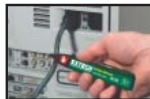
Locate power cord breaks
