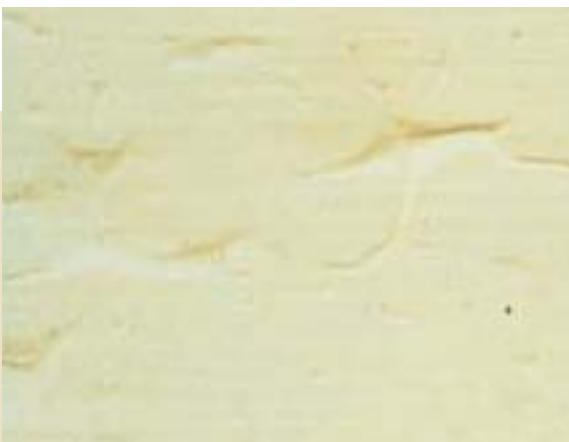
Wrinkling (courtesy Behr/Rohm and Haas).
